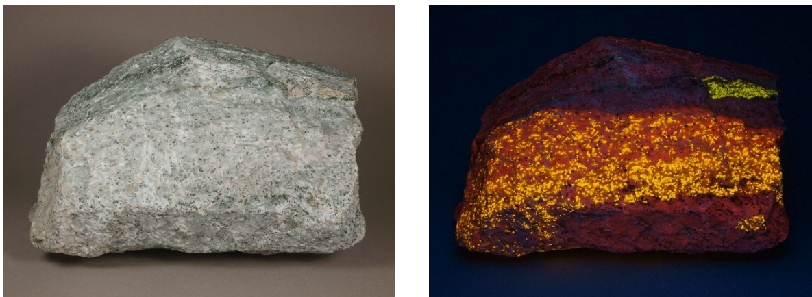
Figure C3. Wollastonite from the 700 level of the Sterling mine, viewed under normal light (left) and shortwave ultraviolet light (right). Note the sharp change from yellow-fluorescent wollastonite in the lower part of the specimen to orange-fluorescent wollastonite above. Sterling Hill Mining Museum specimen, 26 x 17 x 10 cm.
