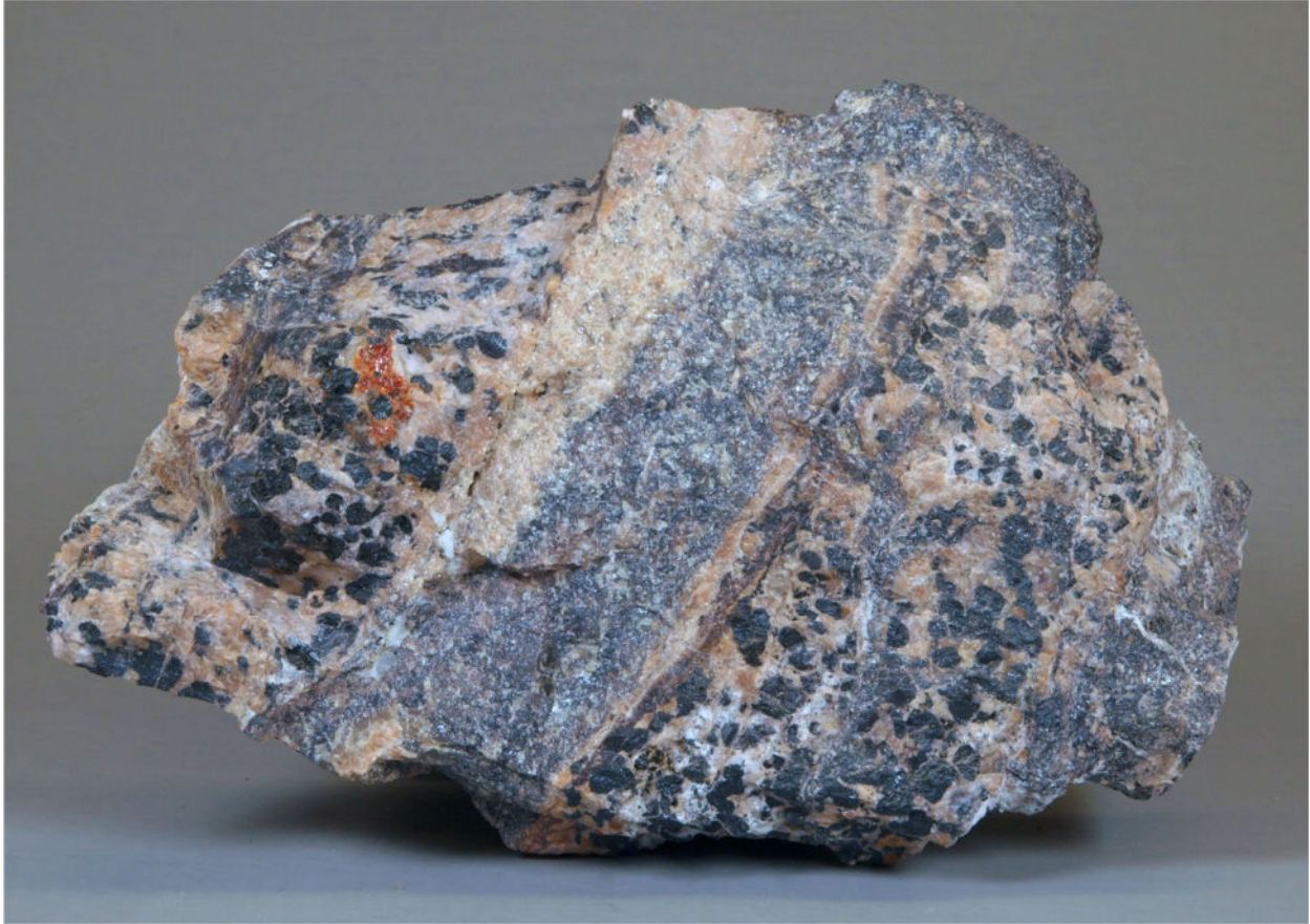
Figure C8. A sample of faulted, hydrothermally altered, zincite-depleted ore cut by a fault lined with gray to tan sphalerite from 970 stope, 1000 level. The ore contains much secondary hydrothermal willemite in microscopic grains that fluoresce bright green SW. Specimen size is 14 x 9 x 3.5 cm.
