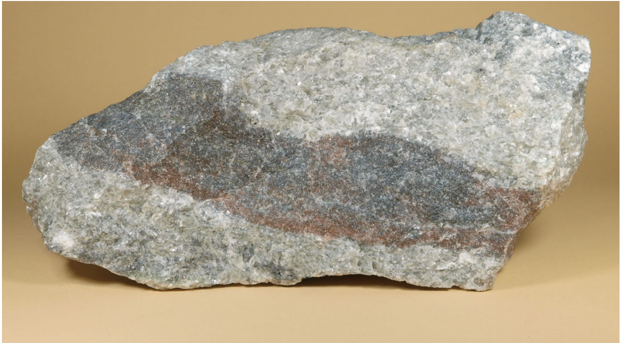
Figure C5. A large specimen of zinkenite (dark gray) and realgar (brownish-red) in pale gray calcite marble. Additional minerals in the zinkenite-realgar layer include fine-grained quartz, sphalerite, pyrite, and arsenopyrite. This sample was collected on 900 level, from a downdip continuation of the 800-level zone described here. Franklin Mineral Museum specimen FMM-2639, 31 x 14 x 7 cm.
