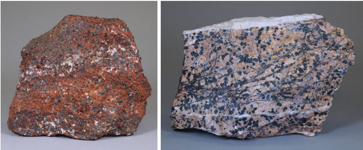
Figure C7. Left, high-grade zincite-franklinite ore from 970 stope, 1000 level of the Sterling mine. Right, similar ore from the thrust-fault zone, where the zincite has been removed by hydrothermal fluids and reprecipitated along the faults as secondary sphalerite and willemite. The granular black mineral in both specimens is franklinite.
