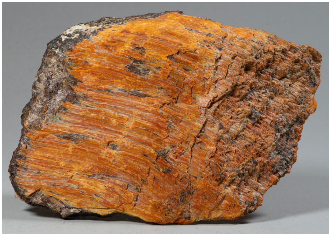
Figure 2. Sheeted mass of fibrous to splintery zincite on a fault surface in high-grade, franklinite-zincite ore. Each zincite fiber is rooted to the wall rock along the left side of the specimen and is broken on the opposite end. The small steplike fractures produced by breakage of the fibers face to the right in this view, indicating the missing fault block moved in that direction. Franklin Mineral Museum specimen FMM-7909, 11 x 9 x 6 cm.
