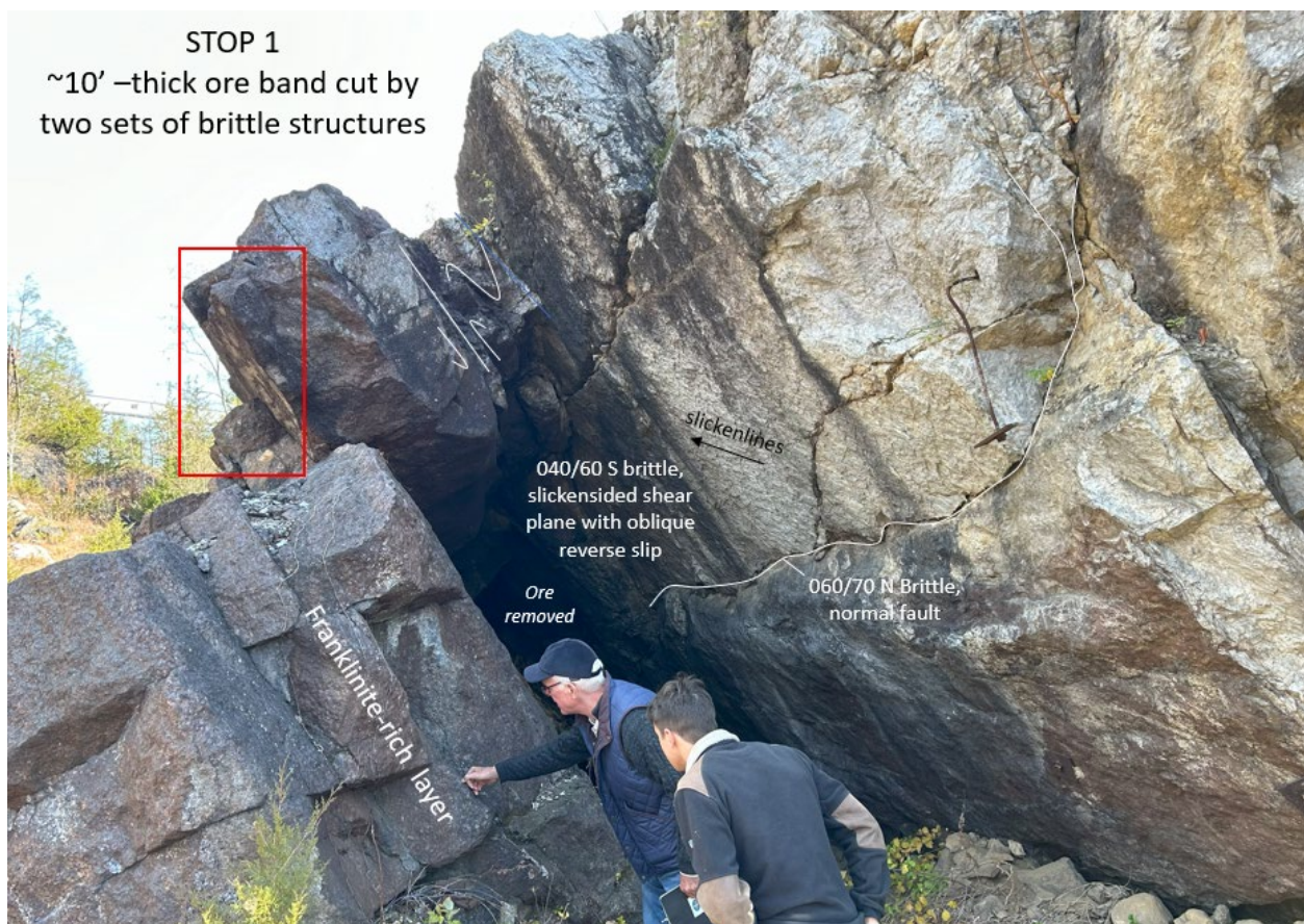
Figure 8. A short (~5 meter) drift in the east layer removed about a 2-meter ore section. The thick, basal franklinite-rich layer was not mined. A red box in the left middle highlights the underside of an infiltrated layer shown in figure 9. White annotation on the hanging-wall fault planes denotes their structural orientation. Small folds can be seen high on the rock bridge above the drift.
