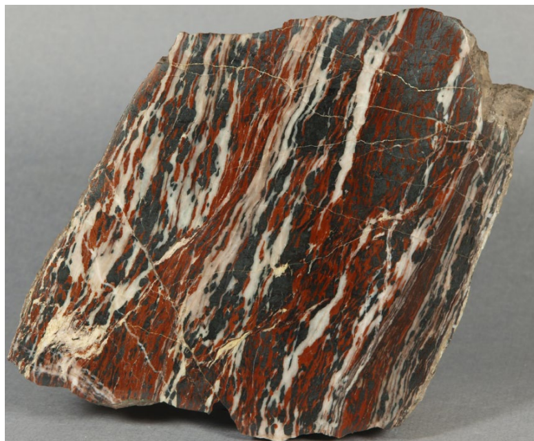
Figure 9. Mylonitic fabric in willemite-franklinite-calcite zinc ore from the Nason fault, 1250 stope below 700 level, Sterling mine. Sterling Hill Mining Museum specimen SHMM-1367, 13 x 12 x 7 cm. The visible surface is sawn and polished. Hundreds of specimens of this material were produced from this stope and sold to collectors. The willemite fluoresces green and the calcite red under shortwave ultraviolet light.
