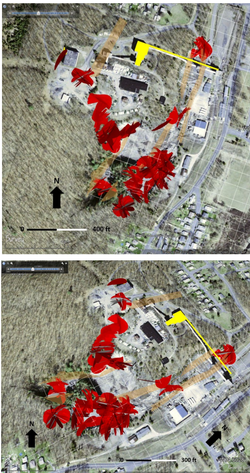
Figure 34. A 3D plot of 308 fault planes mapped at Sterling Hill near ground surface by Verbeek and Grout (Chapter 3) on a 2002 aerial image in GE Pro. Each red ellipse is scaled at 10-m strike and 6-m dip length (5:3 aspect ratio). The symbols were generated using WGS84 geographic latitude and longitude coordinates and structural dip /dip azimuth notation. The top diagram is a map whereas the bottom view is tilted and rotated clockwise. Further refinements can include variable scaling of smaller and larger faults. The yellow building is a reference building for aiding in geolocation of the associated 3D CAD model that was imported into GE as a Collada (*.dae) object model (fig. 32). The light orange stripes are the ore layers projected to ground surface.
