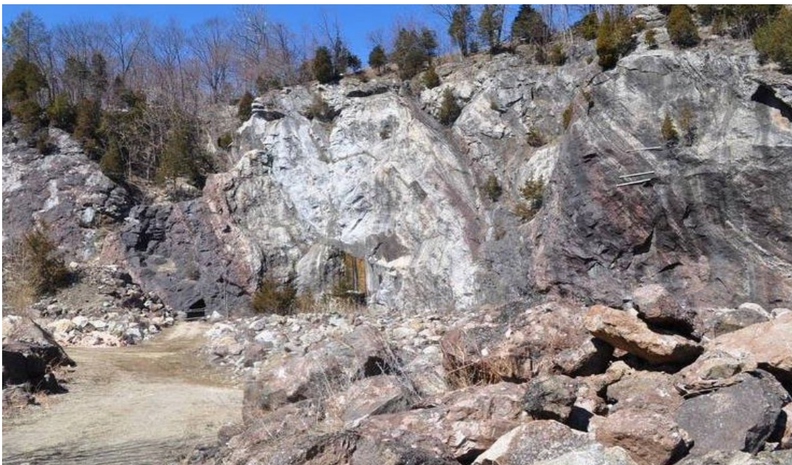
Figure 6. The southern surface exposure of the Sterling Hill Passaic pit illustrating the ore zones of figure 4 beginning with the "white limestone" at the center surrounded by the "brecciated gneiss"; "pyroxene limestone"; and "brown and black willemite" zones.
