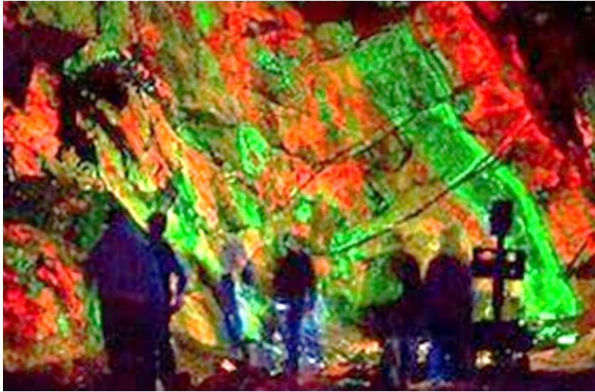
Figure 14. Steeply dipping layers (2.5 m thick) of coarse-grained, graphite-free marble (red) and willemite – franklinite ore (green) on the right have been converted into shapeless blobs of willemite – franklinite ore in a matrix of fused carbonate on the left. Photo is modified after Barberia (2016).
