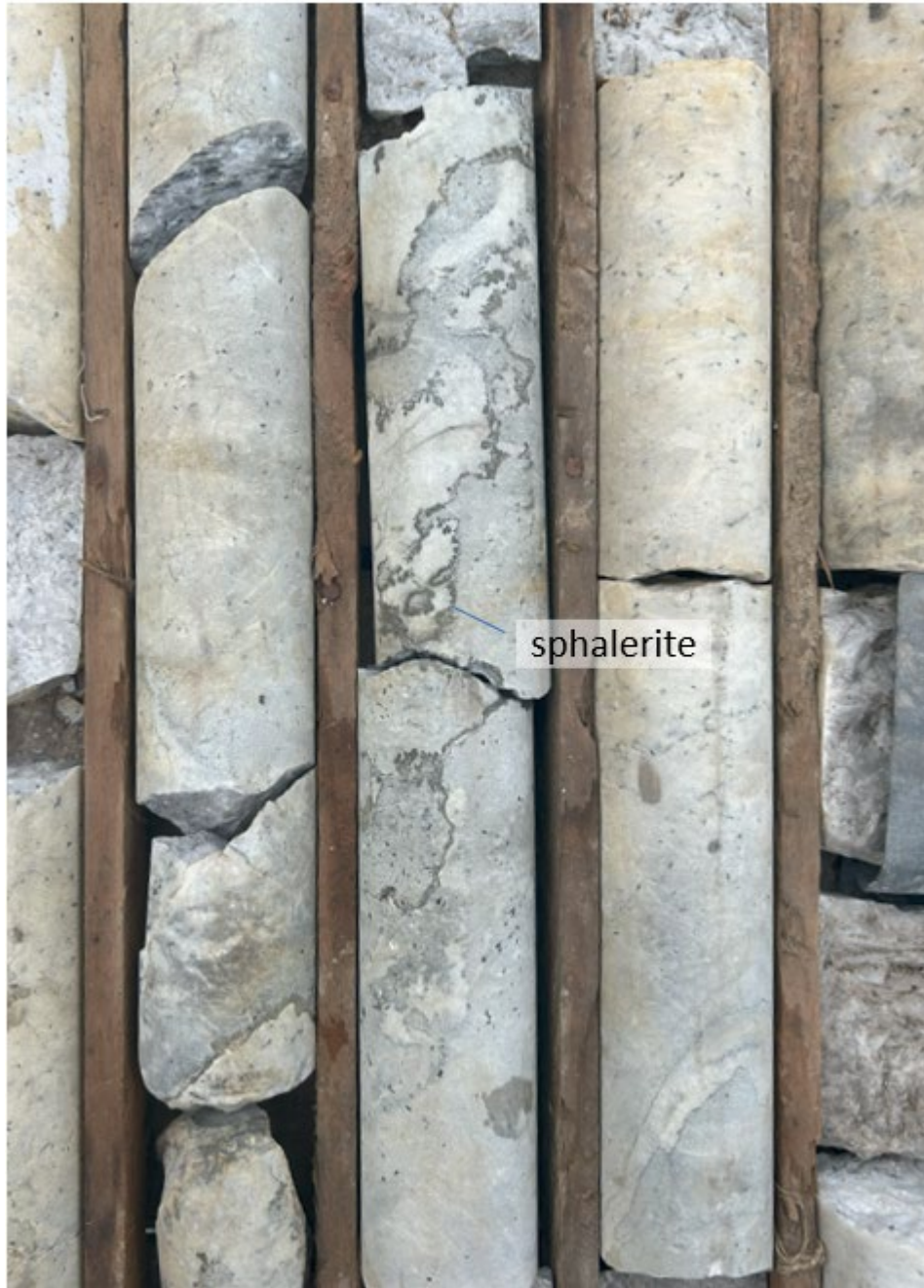
Photograph of sphalerite deposited along hydrothermal solution fronts in core DDH S-262 around the ~1883 ft section. Please see chapter 2, figure 12 for how this section correlates with the Sterling Hill ore body. The core is held in the Rutgers University core repository.
