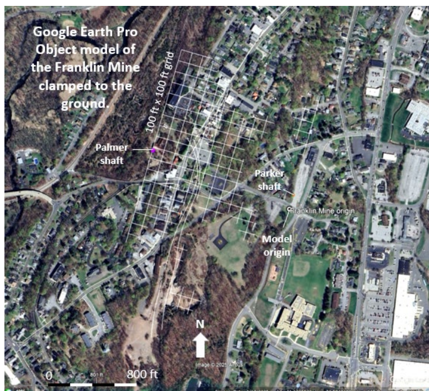
Figure 32. Map (top) and oblique, north view (bottom) of part of the Franklin Mine model that was added to a GE KMZ file as a Collada object (dae file). The map view has the model clamped to the ground. The north view shows the model raised 400 meters (~1312 ft) vertically above ground. This object model includes the mine grid, some multicolored stope sections, and line projection of the ore body to the surface.
