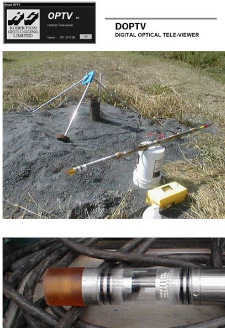
Figure 8. An optical televiewer or optical borehole imaging tool generates a photographic scan of the borehole. The older (left) and newer (right) optical-imaging probes (OPTV and OBI) used by the NJGWS.
