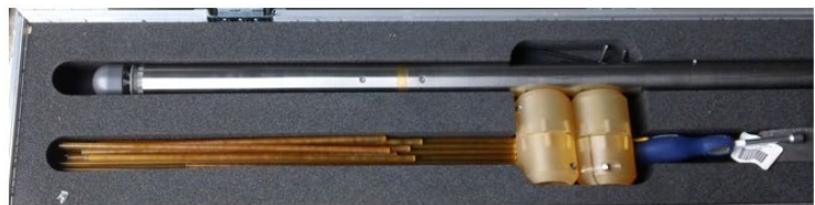
Figure 8. An optical televiewer or optical borehole imaging tool generates a photographic scan of the borehole. The older (left) and newer (right) optical-imaging probes (OPTV and OBI) used by the NJGWS.
