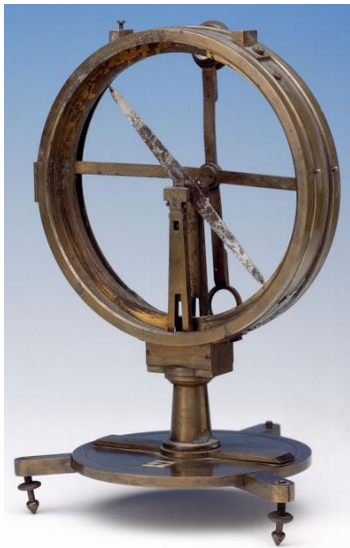
Figure 3) Typical magnetic dip meter used in late 1800s.
