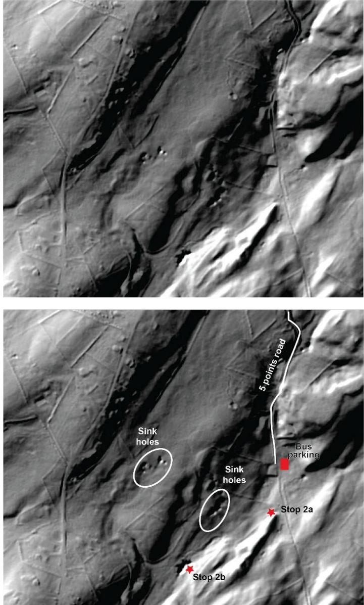
**Figure 2.1:** Lidar images of the area around Stop 2. Red symbols identify the location we will depart the bus, the exposure of the dolomite described in Stop 2a, and the location of the active sink in Stop 2b. The series of sinkholes near the center of the photo marks the approximate location of the Martinsburg – carbonate contact. Another set of sinkholes occurs to the east southeast.
