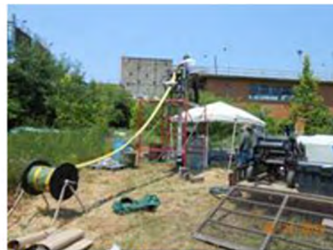
FLUTe liner hydraulic conductivity test of 68BR NAWC
