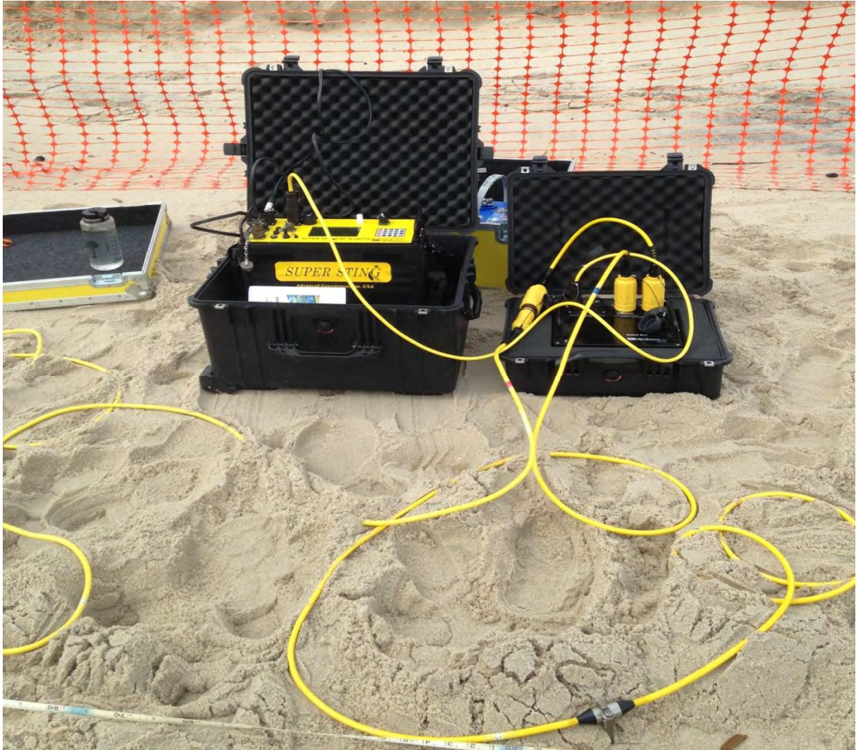
Figure 2: AGI Supersting Resistivity unit with 84 electrode switchbox.
