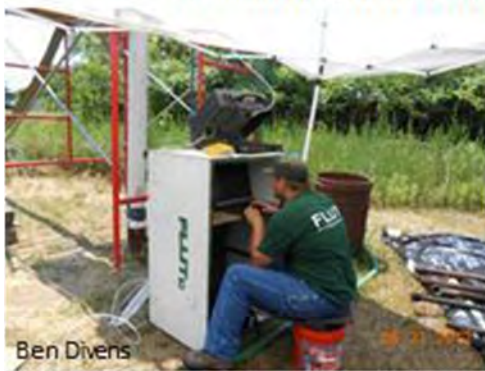
FLUTe liner hydraulic conductivity test of 68BR NAWC
