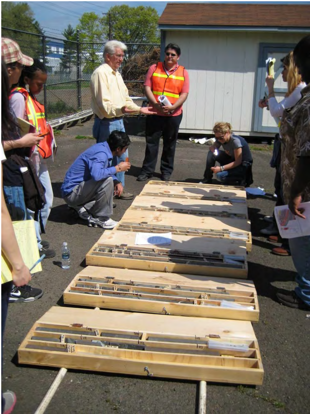
Figure 7: Rock core used to research and teach about NAWC site geology and hydrogeology. Professor Lampousis and students from City College of NYC.
