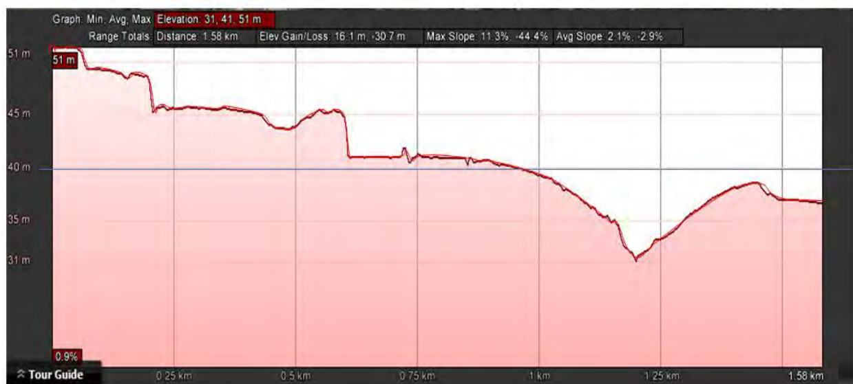
Figure 23: Google Earth (GE) was used to develop cross-section elements including a topographic profile (bottom graphic) that was auto-generated along the section trace (top A-A'). The profile topography requires further manipulation to place it into the project with the proper aspect because it is not captured with equal horizontal and vertical scales (1:1 scale). The deviation between dip azimuth and the section trace is highlighted in A. simply screen captured, pasted into MS PowerPoint (B.) and then traced using a freeform polyline. Note that when using GE to generate a topographic profile, that the resulting image is a scale other than 1:1
