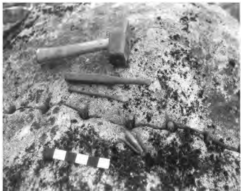
Figure 3: Plug and feather tools used to harvest building stone (Gage and Gage, 2005).
