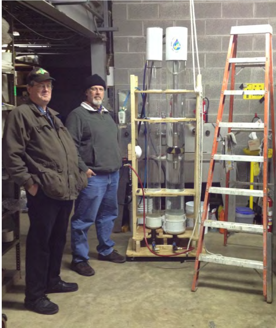
Chief James T. Boyle and coauthor Mark French oversees HFM system testing in the NJGWS garage. The HFP-2293 is positioned in the clear, 7.5-inch pipe to the right and setup for upward, low-flow testing.
