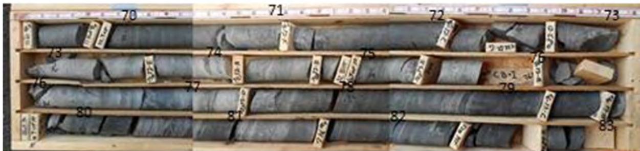
Figure 10: Rock core containing massive and disseminated sulfide minerals where abiotic TCE degradation occurs.
