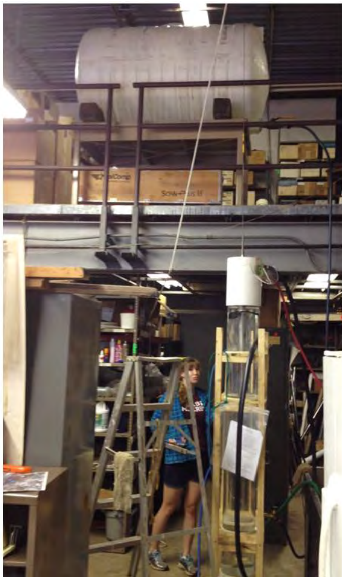
Figure 8: A 250-gallon plastic tank lofted about 8-ft above the testing apparatus provided a steady water supply needed for low-flow testing. Ms. Rachel Filo attends to the flow apparatus during testing.
