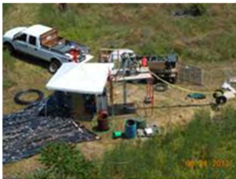
FLUTe liner hydraulic conductivity test of 68BR NAWC
