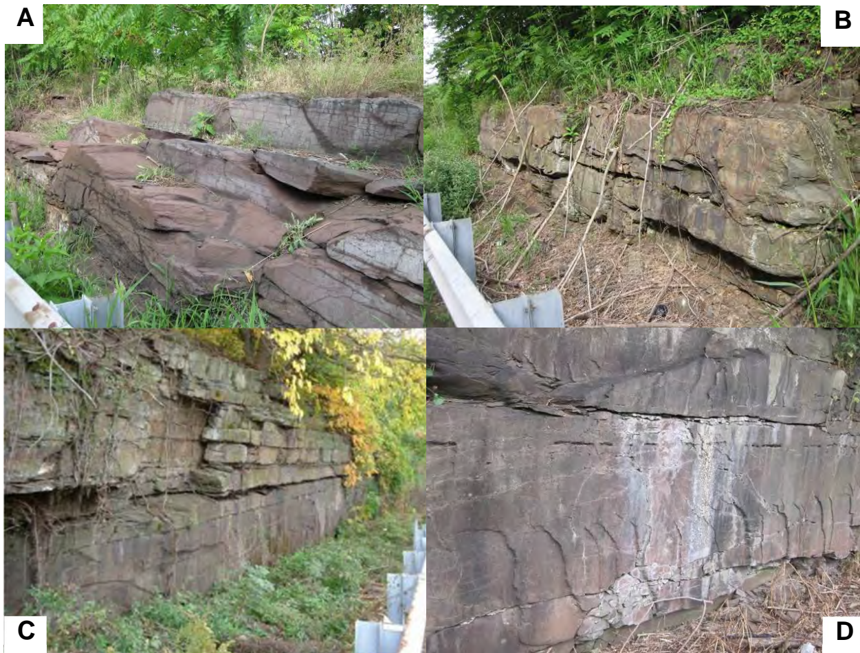
Figure 1: Road cut exposure of upper part of Prahls Island Member of Lockatong formation showing: (A) chemically altered micro fractures, (B) differentially weathered strata of Van Houten cycles (C) Strata bound joints and fissile and indurated strata, and (D) punctuated flow in a water bearing fissile strata.
