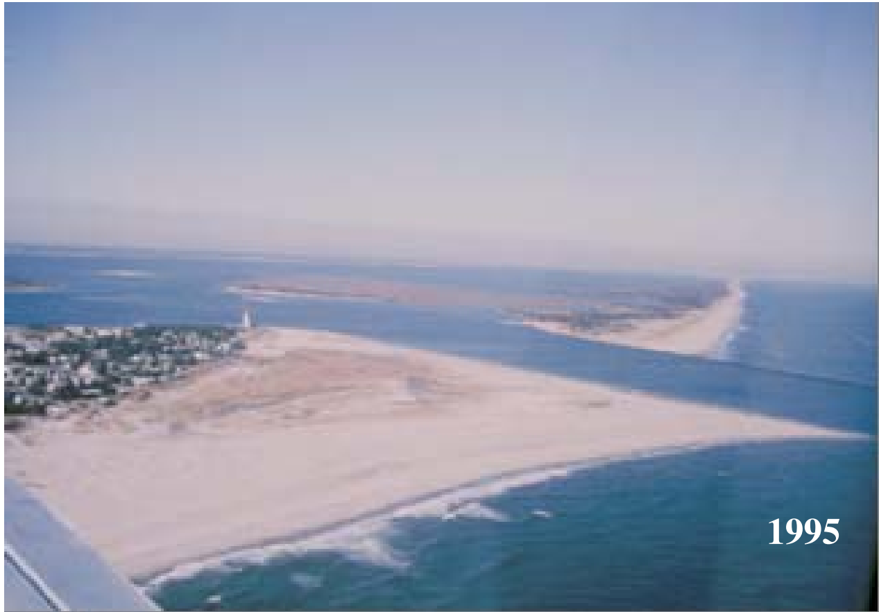
Figure 1B. By 1995 the new jetty was complete and the sand was accumulating along the south side of the south jetty to create what we see today. The dunes and vegetation will change slowly over time into a maritime forest that should protect Barnegat Light Borough for decades into the future (photo-S. Farrell, 1995).
