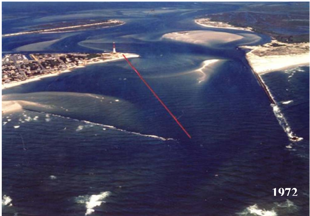
Figure 1A. 1972 view of Barnegat Inlet showing the original “arrowhead” design for the inlet jetties. Note the emergent shoal in the center of the inlet. One could leave the inlet one day with the navigation channel along the south margin only to find it along the north margin when you returned two days later. The red line approximates the location of the 1990 reconstruction of the south jetty. No old jetty rocks were removed, simply became buried in the fillet that deposited (photo-S. Farrell, 1972).
