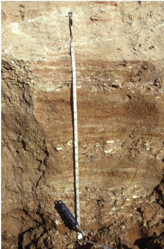
Figure 8: Silty fine- to medium-grained sand with intercalated beds of light- to dark-colored clayey silt of the Sayreville Sand in the former Sayre & Fisher Company clay banks in Sayreville, NJ. The measured section from the top of the tape measure to the spade is 3.75 feet (1.1 m).
