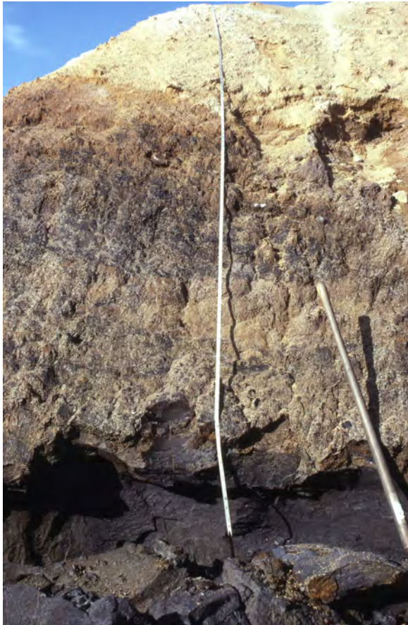
Figure 6: Exposure of the Woodbridge Clay overlain by the Sayreville Sand in the former Sayre & Fisher Company clay banks in Sayreville, NJ, now lost to the TowneLake housing development. Note the undulating contact between the two units. The measured section from the top of photograph to the end of the tape measure is 10.5 ft (3.2 m).
