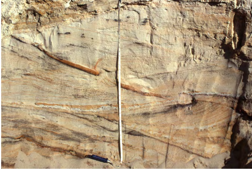
Figure 7: Stacked trough cross-beds with pronounced internal lamination of the Sayreville Sand in the former Sayre & Fisher Company clay banks in Sayreville, NJ. The measured section from the top of photograph to the spade is 4 feet (1.2 m).
