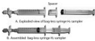
New syringe diffusion sampler for hydrogen gas: *Ground Water* journal article by [Vroblesky and others, 2007](#).
