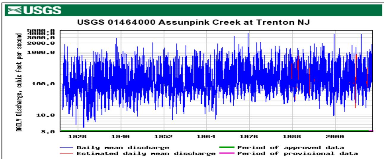
Discharge measurements for the stream gaging station on the Assunpink Creek in Trenton
