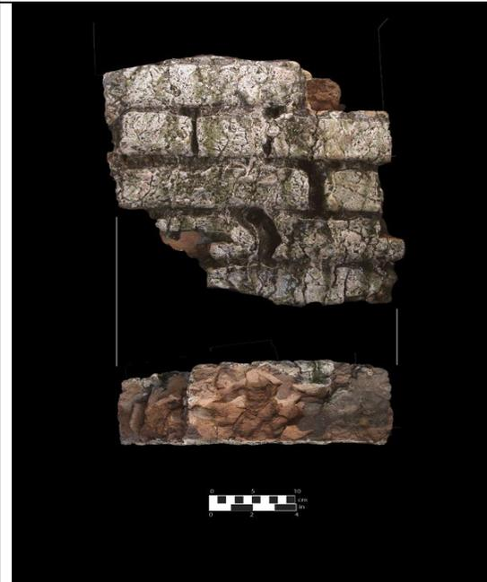
Brick from furnace with face melted to glass
