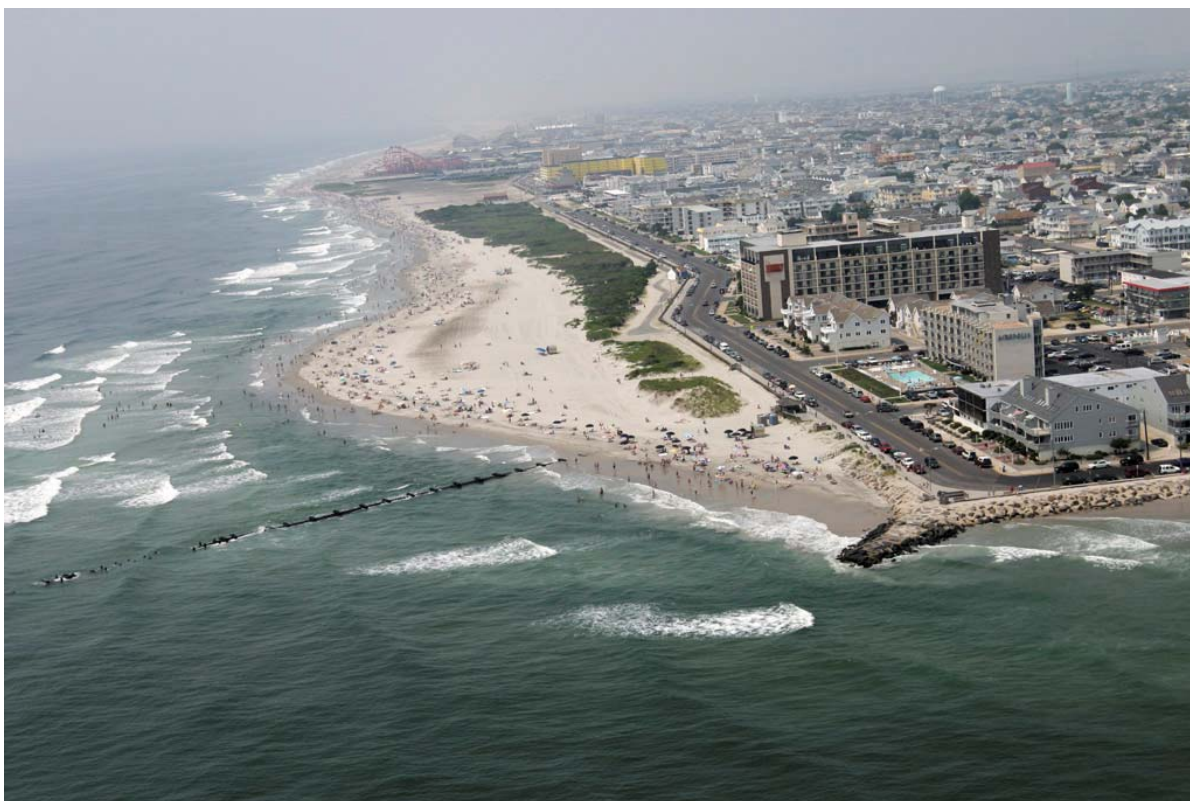
Figure 2. The beach at the City of North Wildwood in 2004 as changes to the Hereford Inlet ebb-tidal geometry were changing to produce a loss of sand from the bulge in the beach above to move material south into Wildwood and north into Hereford Inlet.
