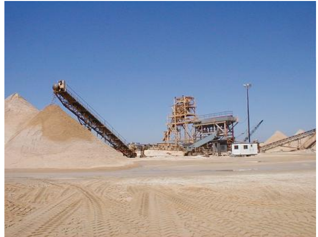
Figure 18. Dredging operation and sand washing of Cohansey sand Cape May County.
