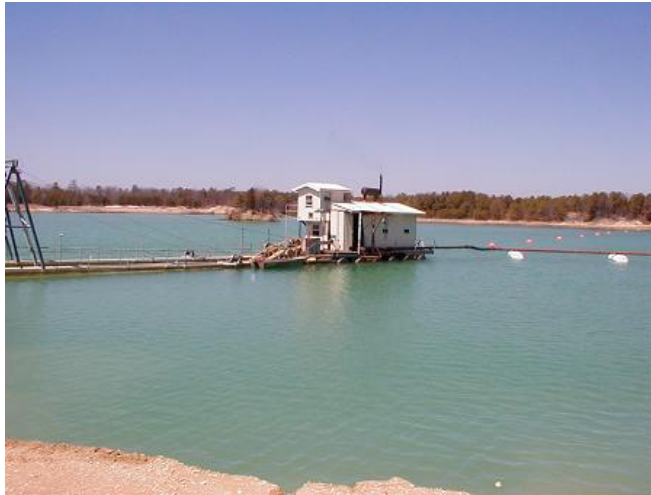
Figure 18. Dredging operation and sand washing of Cohansey sand Cape May County.
