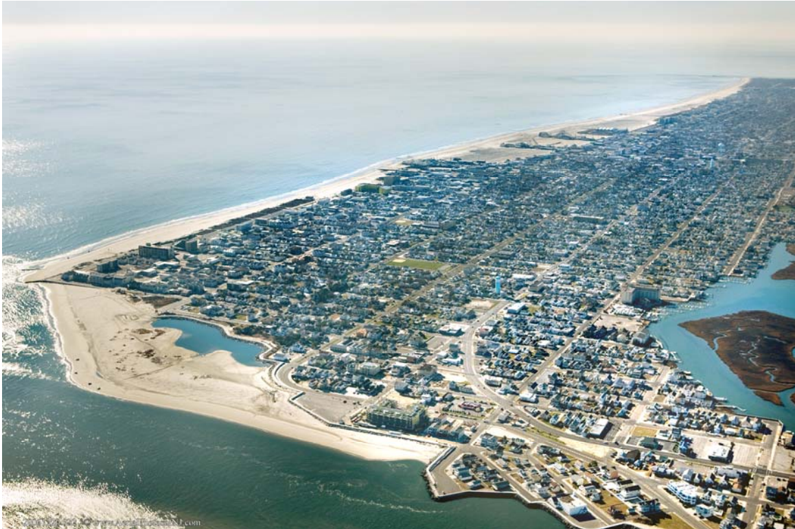
Figure 3. North Wildwood in 2008. Note that the bulge is gone, the shoreline has retreated, but massive quantities of sand have moved to the Hereford Inlet shoreline. This is a 25 to 30 year cycle that last occurred in 1962 to 1970.
