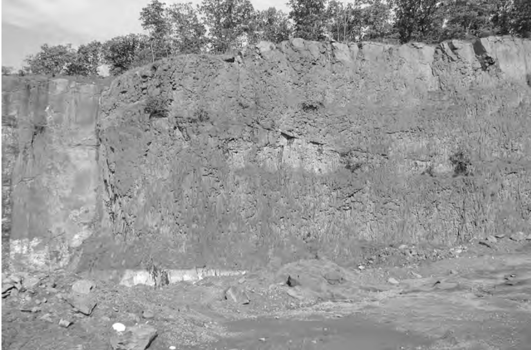
Figure 5. A lava pause exposed as a low angle discontinuity along the middle of the wall, UBC quarry.
