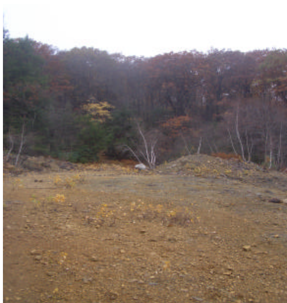
Figure 2. Phillips Mine: Coarse to fine-grained tailings in the foreground. Sparse vegetation is present on the tailings but spatially distributed.
