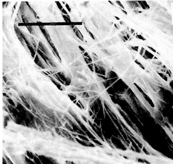
Figure 2. Scanning electron photomicrograph of asbestiform tremolite forming through weathering of prismatic tremolite from the Southdown (Limecrest) Quarry in Sparta (from Figure 3, Germine and Puffer, 1989a). Bar scale equals 10 microns.
