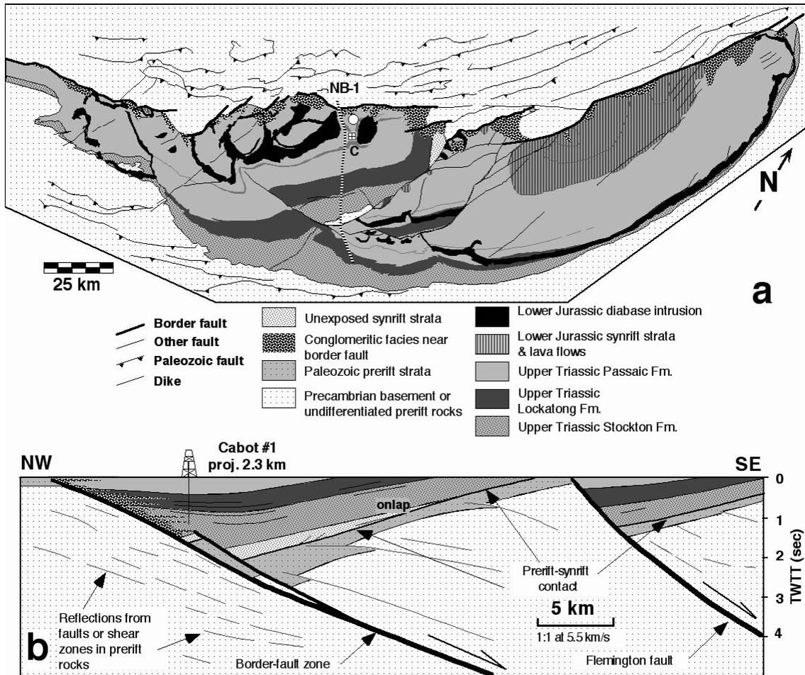
**Figure 3.** (a) Geologic map of the Newark basin showing location of the NB-1 seismic-reflection profile, the Cabot #1 well (C), and the Haycock Mountain outcrop (circle). (b) Interpretation of line NB-1 constrained by surface geology and the nearby Cabot #1 well. Modified from Schlische and Withjack (2005).
