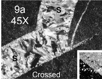
Figure 9a. S1 and S2 albite-filled veins in gray argillite of the Lockatong
