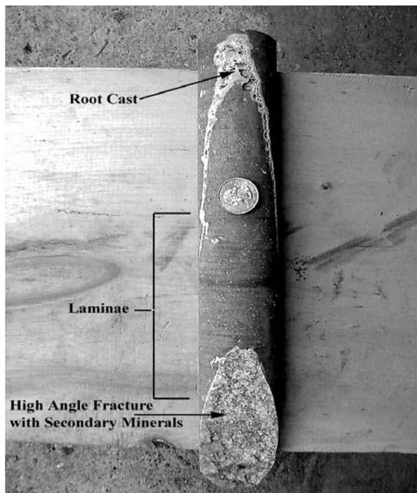
Figure 5. Root casts and banded laminae. The top of this core section represents 63.8 meters below grade. The core width is five centimeters and the quarter is for reference.
