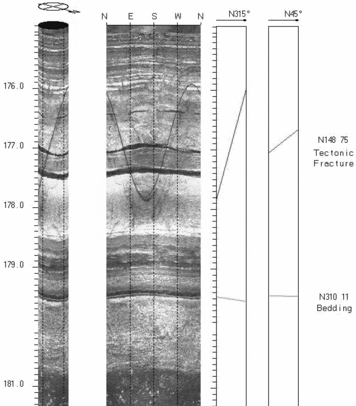
Figure 16. Interpreted OPTV records of borehole walls include a virtual, wrapped-core display (left) and the unrolled borehole image (center). The line diagrams to the right show apparent dips of interpreted structures from two orthogonal perspectives. Annotation on the far right denotes dip azimuths of interpreted features. The interpreted records are generated at 1/12 scale and stored as JPEG digital images for archiving and display.
