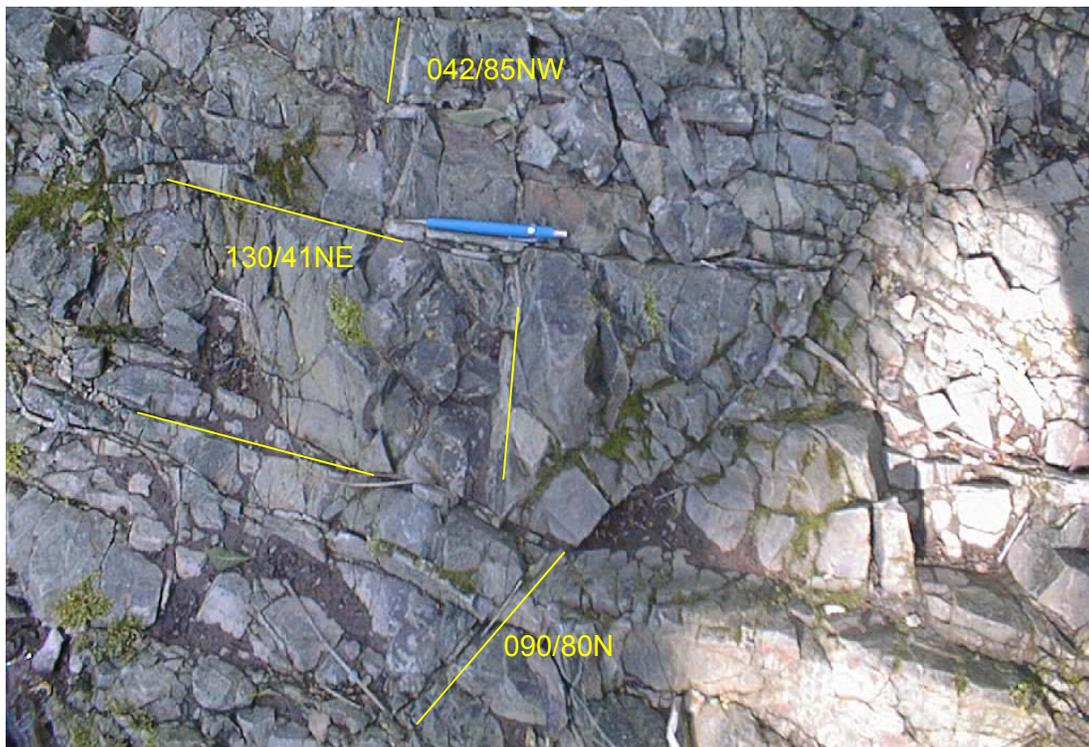
Figure 7. Microcrystalline limestone veins cut the fractured and brecciated basalt at various orientations. Both views are of subhorizontal surfaces in the streambed that stand above water level during periods of relatively low stream flow.
