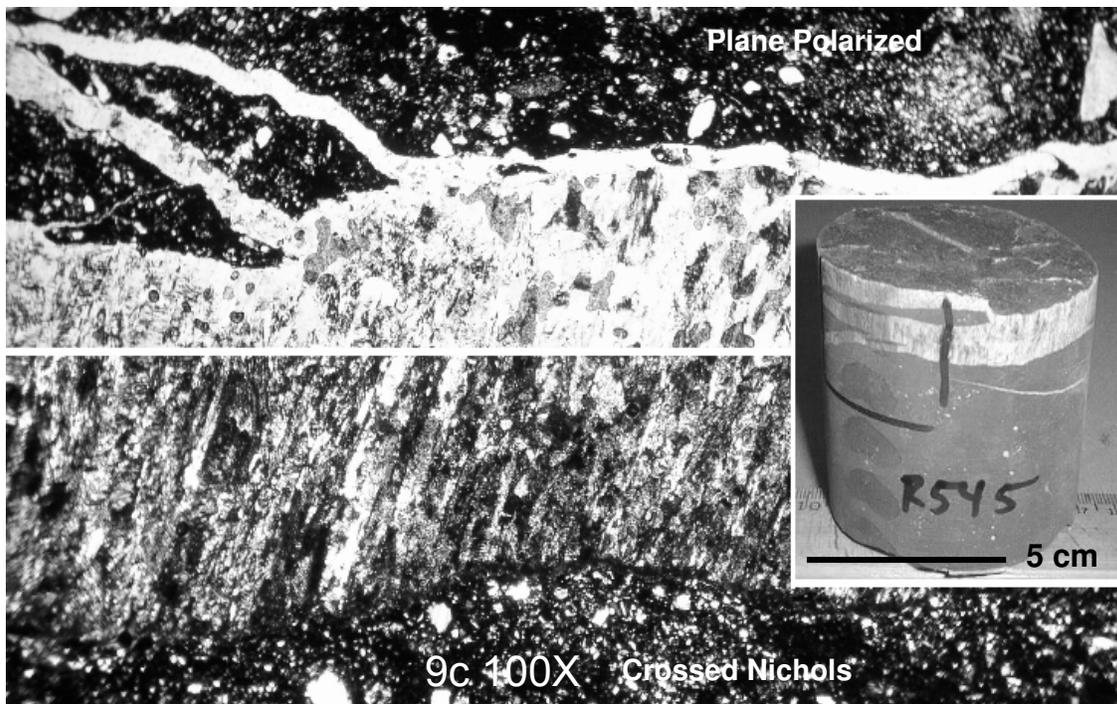
Figure 9c. Gypsum veins are late fillings, mostly oriented sub-horizontal to land surface with sub-vertical crystal fibers. Gypsum veins many centimeters thick are reported from depths exceeding 200 ft in cores from the northeast and central parts of the basin.
