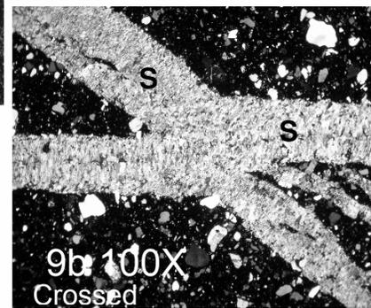
Figure 9b. S1 and S2 fibrous calcite veins in red mudstone of the Passaic Formation, Hopewell Borough, Mercer County
