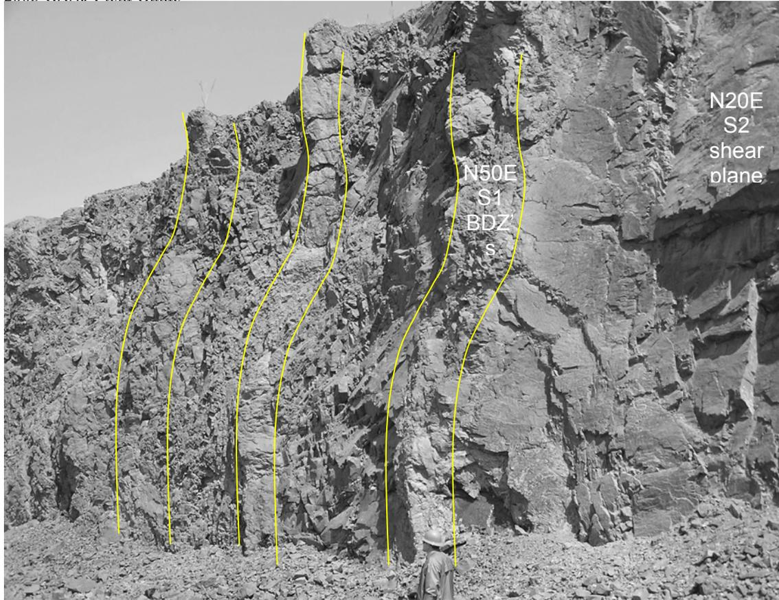
Figure 11. Brittle deformation zones (BDZs) form columnar structures striking parallel to S1 fractures (about N50E) in early Jurassic diabase, Pennington trap rock quarry, Hopewell Township, Mercer County. View facing northeast. The person standing at the bottom center provides a scale.
