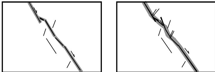
**Figure 1.** Sketch of normal-faulted Passaic Formation at Haycock Mountain (left) and inferred evolution of normal faults (right) based on geometries at Haycock Mountain. From Withjack and Olsen (1999).
