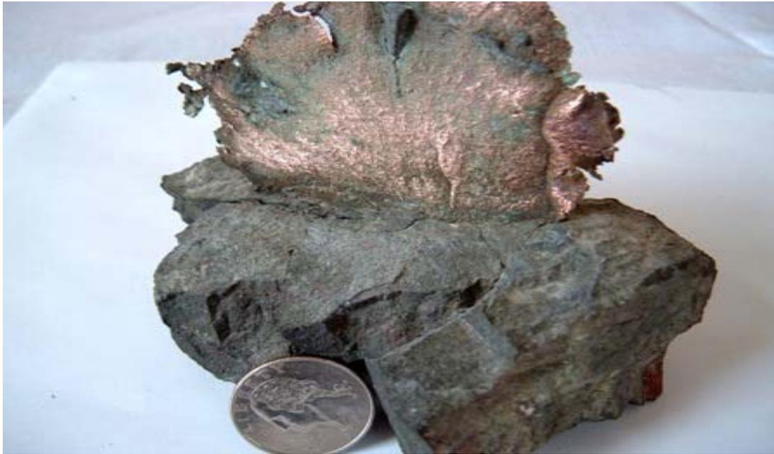
**Figure 8.** Sheet of native copper in basalt joint sampled at Chimney Rock.
