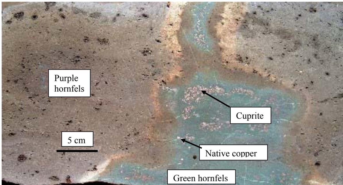
**Figure 6.** Ore sample collected at the American mine consisting of purple, porous, but impermeable hornfels (meta-mudstone) completely devoid of any bedding containing bleached amoeboid shaped structures consisting of green chlorite rich hornfels mineralized with native copper and cuprite with minor chalcocite. Chemical analyses of purple and green hornfels from this sample appear in Table 2.
