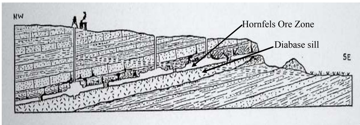
**Figure 5.** Cross section through the Schuyler mine (after Woodward, 1944). The mine workings followed the upper contact of the thin Arlington sill.
