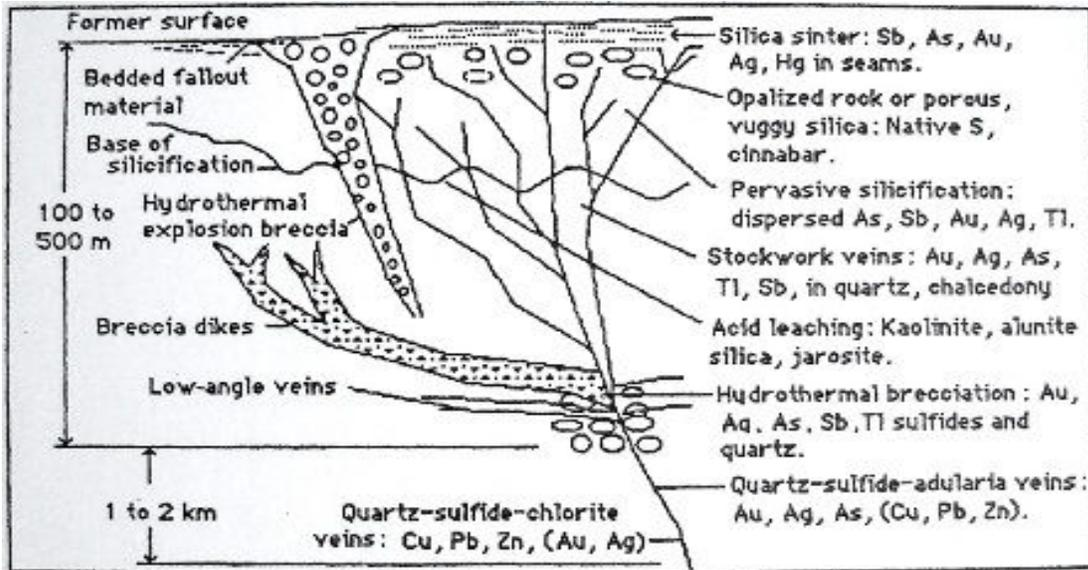
**Figure 9.** Cross section through USGS Hot-spring Model 25a (Cox and Singer, 1986)
