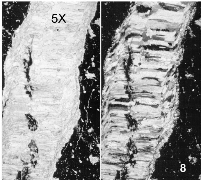
Figure 8c. Other veins have calcite fibers showing localized shearing along fracture walls and vein sutures indicating compressive shearing of earlier fabric. Sample on left shown in plane (left) and polarized (right) light
