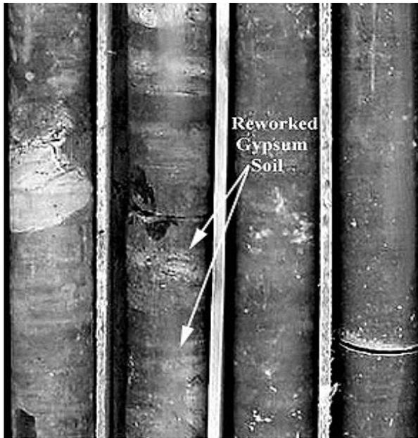
Figure 6. Reworked gypsum soil. Arrowed region was recovered from 82.9 meters below grade. Each core is five centimeters in diameter.
