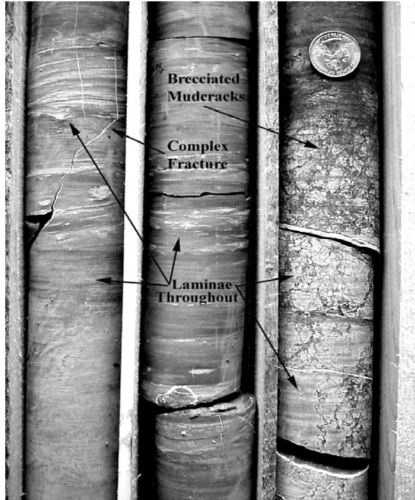
Figure 4. The brecciated mudcracks (right) and complex fracture (left) occur at 38.7 meters and 41.7 meters below grade, respectively. Scale indicated by quarter.
