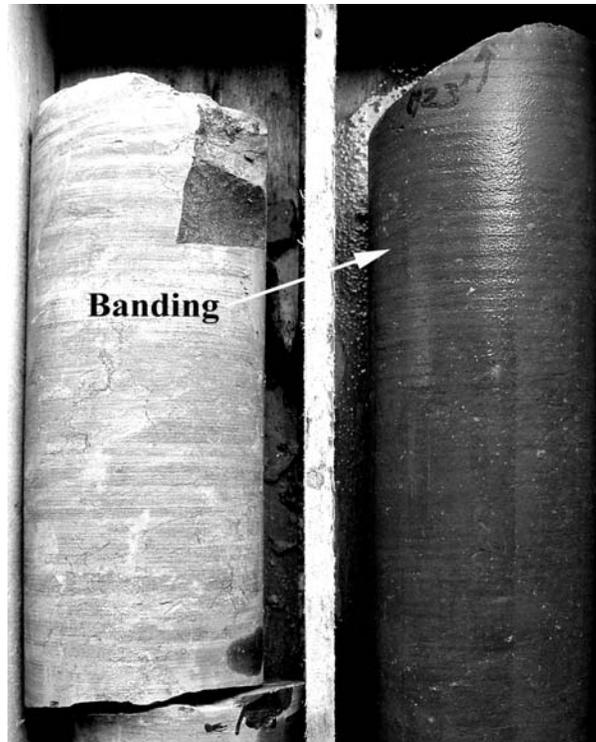
Figure 7. Banding. The cores are each five centimeters in diameter. In this section (37.5 m below grade), approximately 4.4 pairs occur within one centimeter of vertical span.
