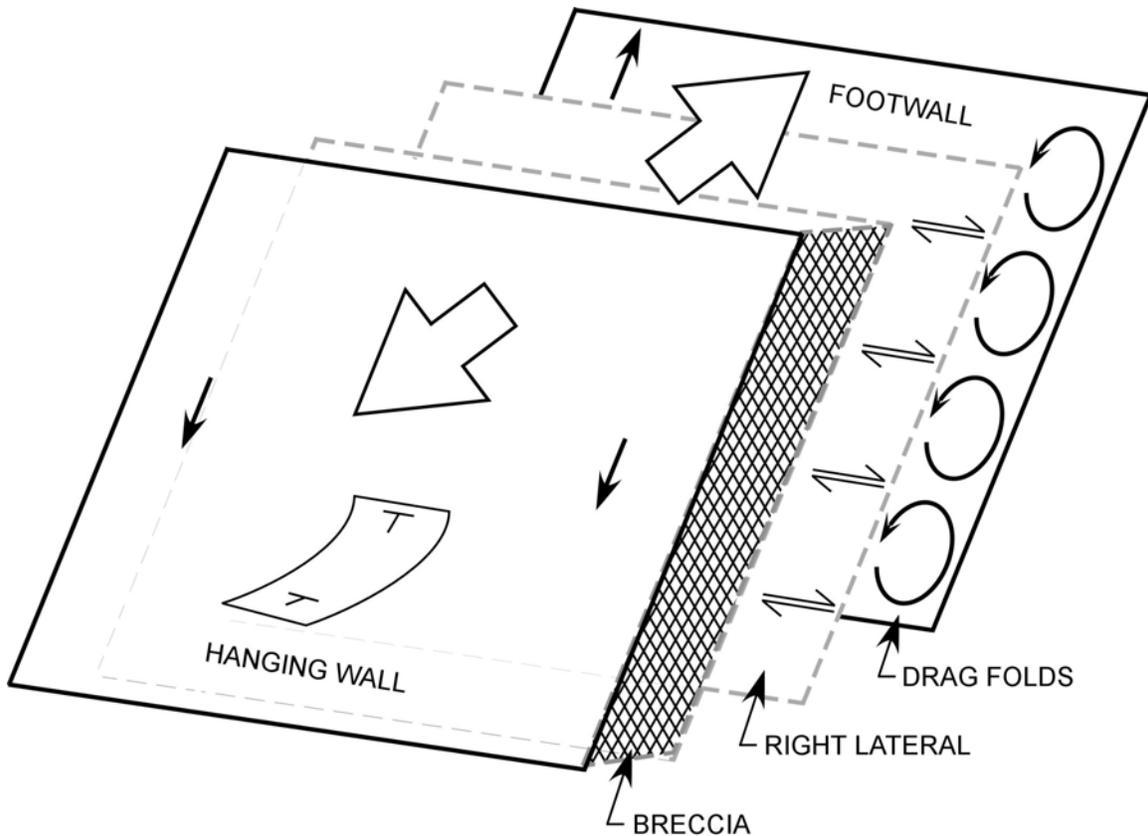
Figure 6. Schematic showing distribution of kinematic structures in the Hopewell shear zone.
