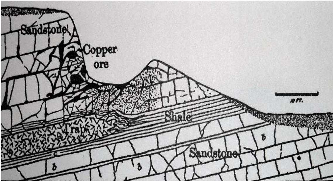
**Figure 2.** Cross section through the Schuyler copper mine (after Darton 1902) illustrating relationship of copper ore to thin veins of fine grained diabase (black) over diabase sill (labeled trap) intruded into Passaic shale. Stippled area at the termination of the trap sheet is explosion breccia.
