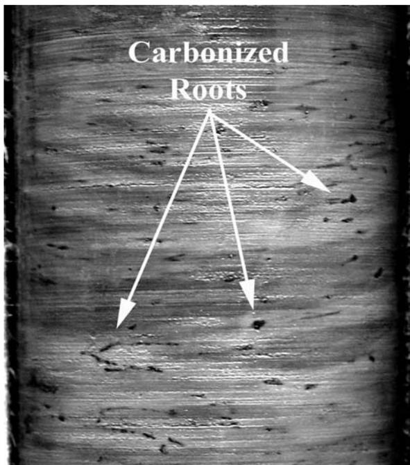
Figure 8. Carbonized roots occur in laminated purple substrate approximately 40.5 meters below grade. The core measures five centimeters in diameter.
