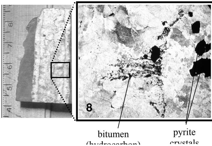
Figure 8b. Some veins are filled with mosaic calcite crystals containing interspersed sulphides (pyrite) and hydrocarbons. Calcite vein in gray mudstone, Rutgers NBDCP core at 2248-foot depth. Vein fillings having multiple suture lines are evidence of ‘crack-seal’ growth (Ramsay, 1980) that give veins a ‘banded’ morphology (Wiltschko and Morse, 2001)
