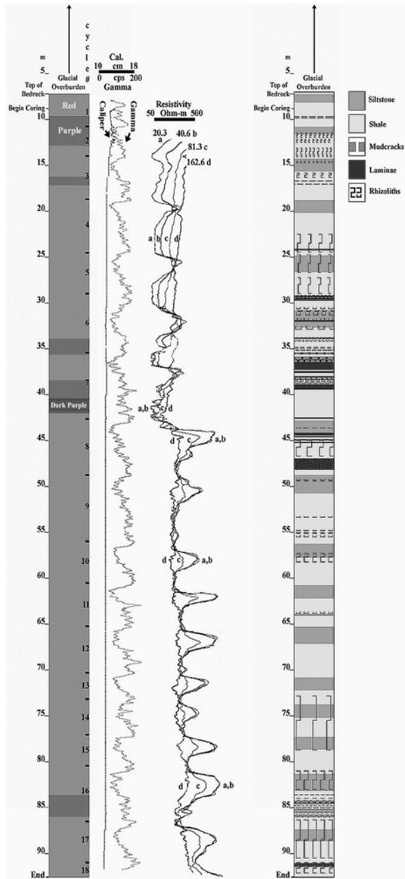
Figure 2. Generalized Geologic Log. Note the change in average grain size recorded in cycle #8 and maintained through cycle #1. Units are as stated.
