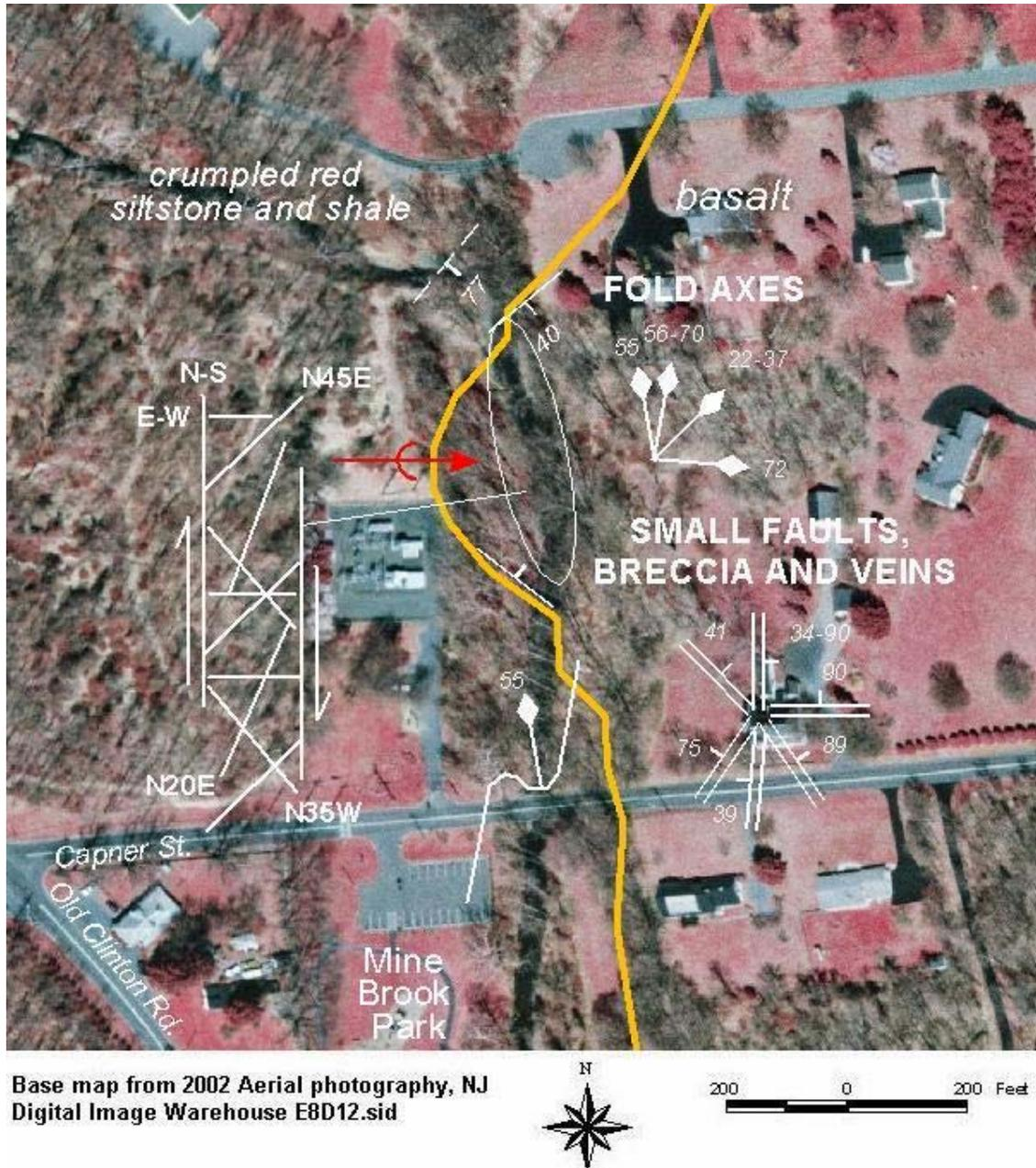
Figure 3. Aerial photograph showing the location and summary of structural fabric exposed in the streambed and banks of Walnut Brook.
