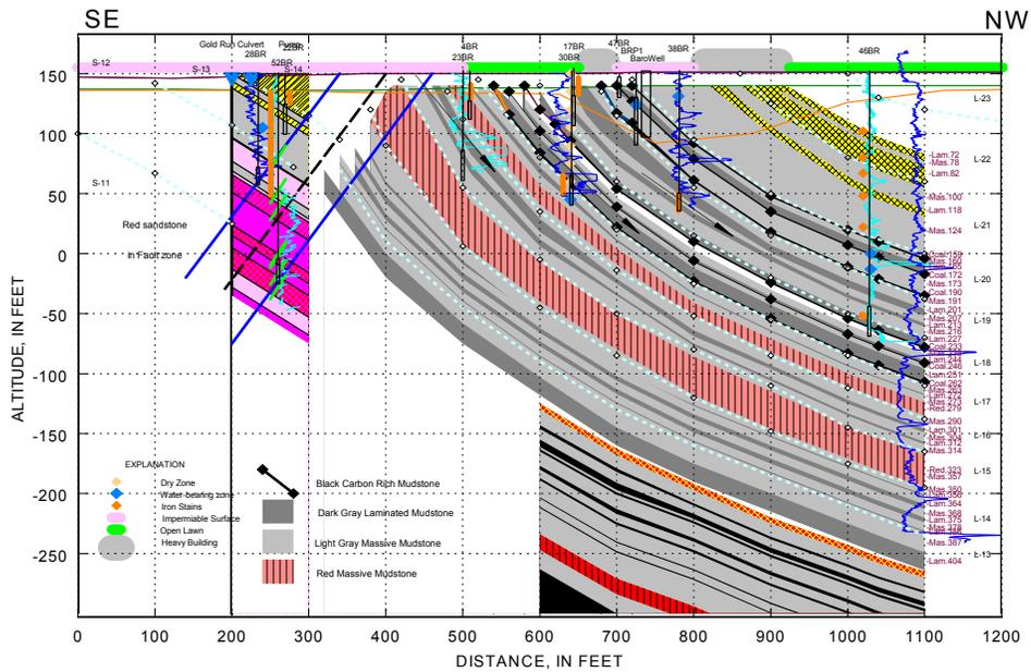
Figure 4. Section through NAWC showing gamma ray stratigraphy and the 42 rock color and nature of the mudstone strata in the Lockatong Formation (modified from Lacombe 2002). Location of the section through NAWC is shown in figure 9.
