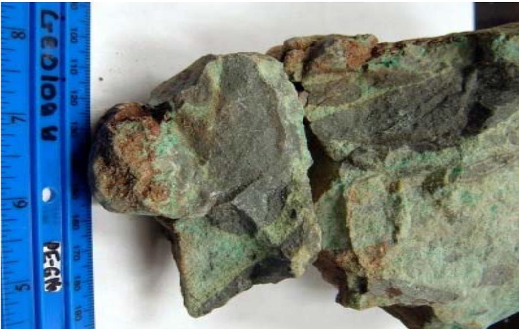
**Figure 4.** Explosion breccia sampled at the Schuyler mine consisting of diabase clasts in copper enriched sandstone.
