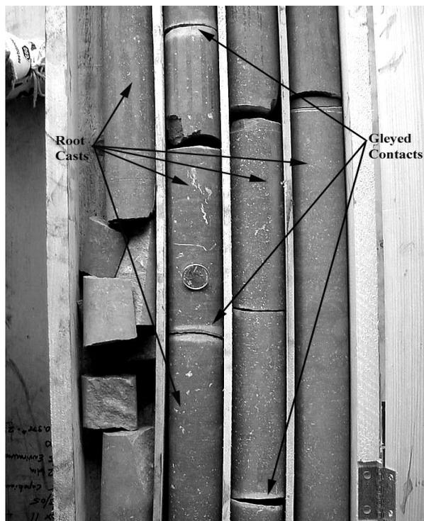
Figure 3. Gleyed staining indicates that anaerobic conditions formerly prevailed along specific fracture zones. The quarter's position corresponds to 59.4 meters below grade.
