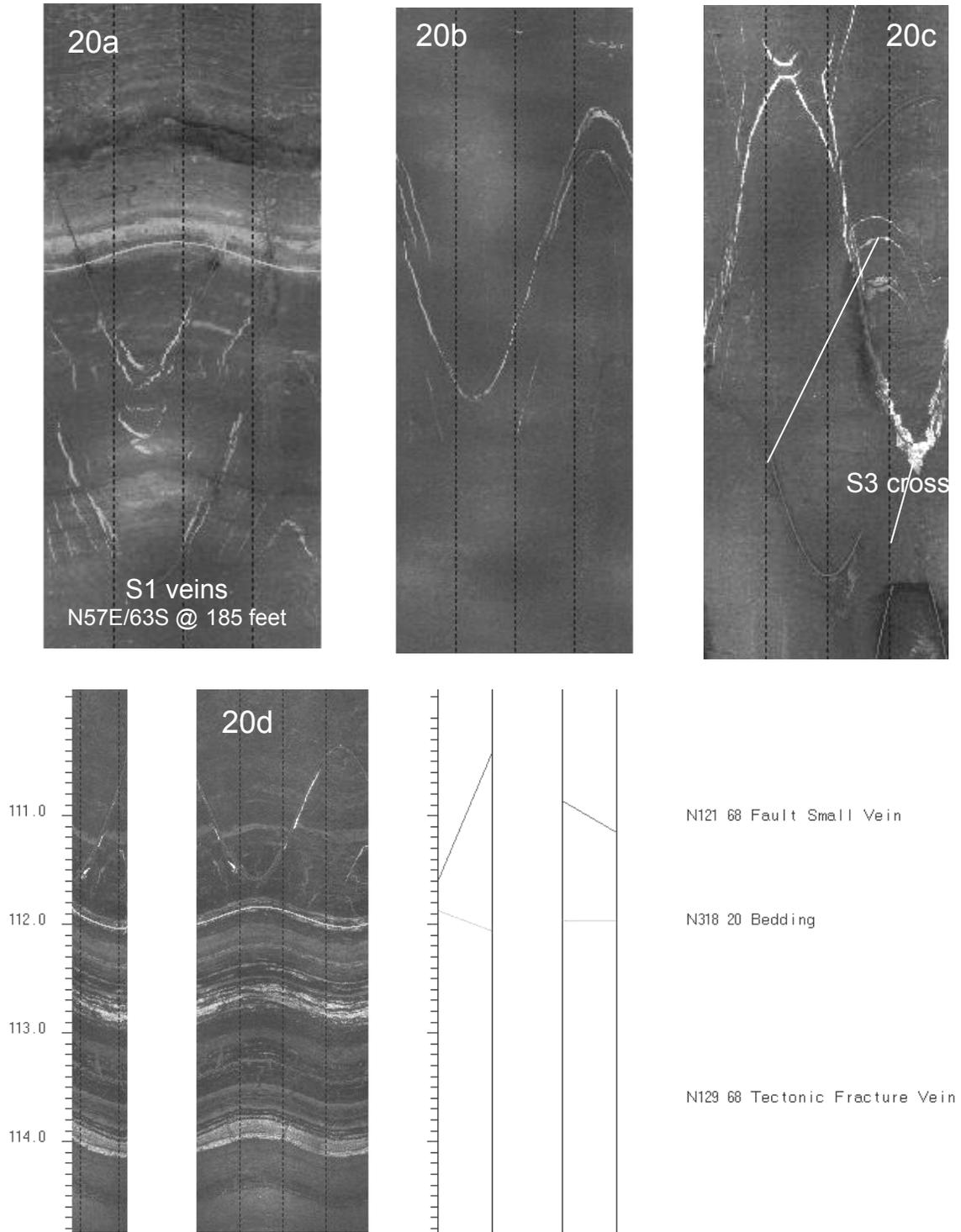
Figure 20. Processed OPTV images showing S1, S2, and S3 vein geometry in red mudstone and gray and black shale in the middle part of the Passaic Formation, East Amwell Township, Hunterdon County. Orientation of images the same as for figure 16. Orientations next to classified structures in the bottom diagram indicate feature dip azimuths. Depth in feet below land surface.
