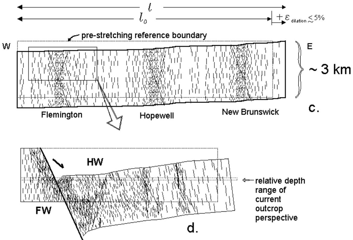
Figure 26. A schematic profile of basin strata showing progressive strain effects associated with the S2 fracture swarms extending from Flemington to New Brunswick, NJ. Location of profile shown in Figure 28.
