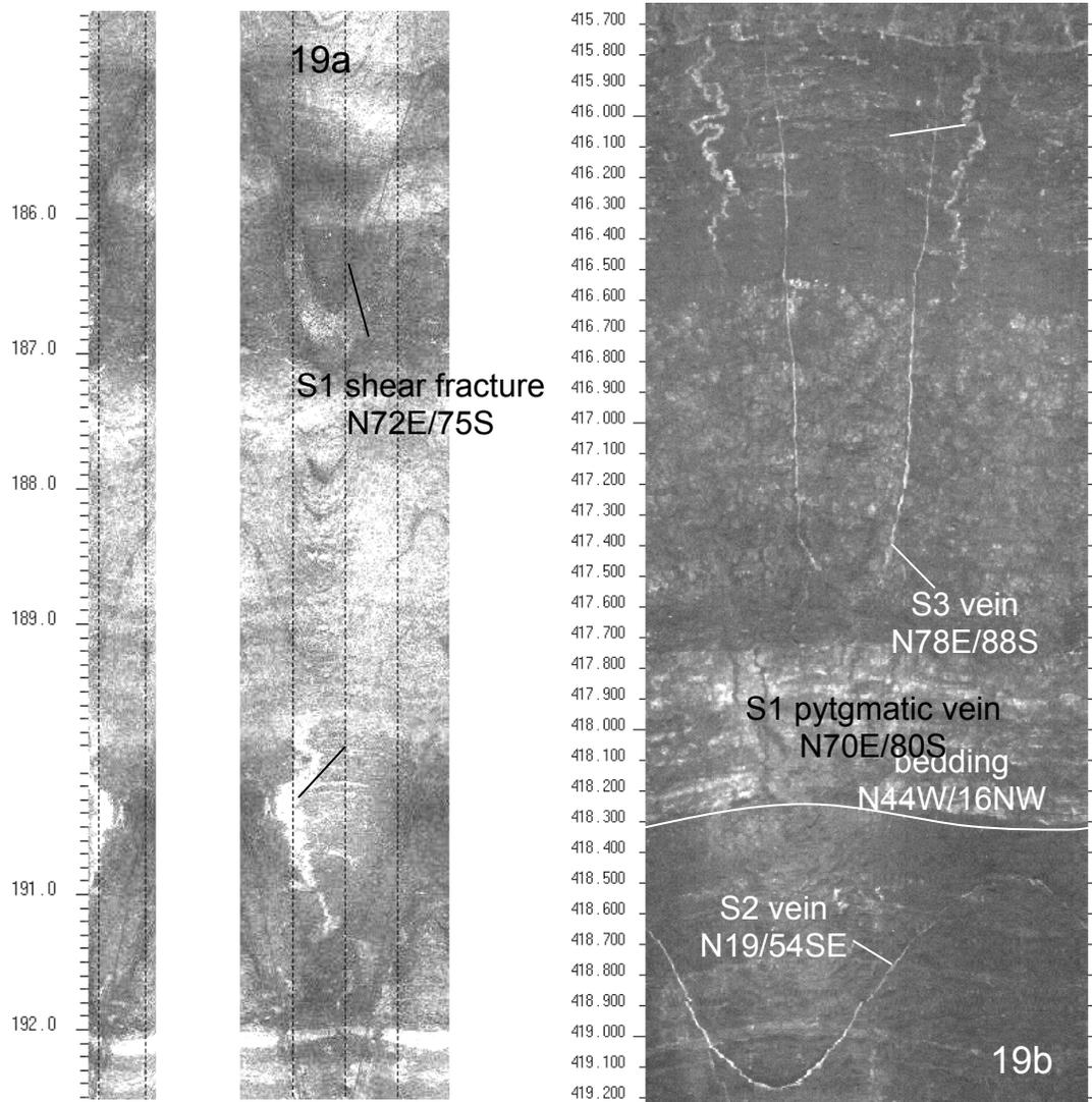
Figure 19. Processed OPTV borehole record (19a) and unprocessed OPTV borehole image (19b) showing examples of S1, S2, and S3 fracture geometry in the Lockatong Formation, Raritan Township, Hunterdon County. Figure 19a shows folded S1 veins and normal dip-slip offset of beds across a S1 shear fracture. Figure 19b also shows a pygmatically-folded S1 vein and later S2 and S3 veins. Orientation of OPTV records the same as shown in figure 16.
