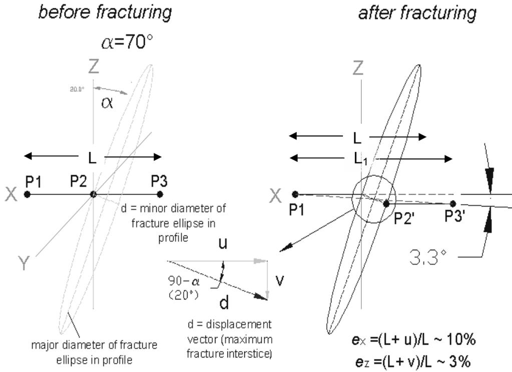
Mode I fracture dipping at angle  $\alpha=70^\circ$
