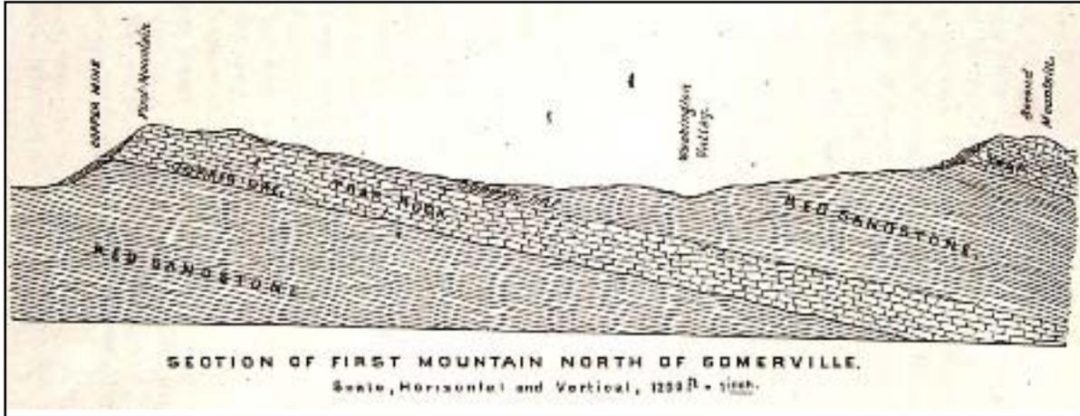
**Figure 7.** Idealized section through copper mines north of Somerville after Lewis (1907) illustrating confinement of ore to the contacts of the “First Mountain” Orange Mountain basalt.
