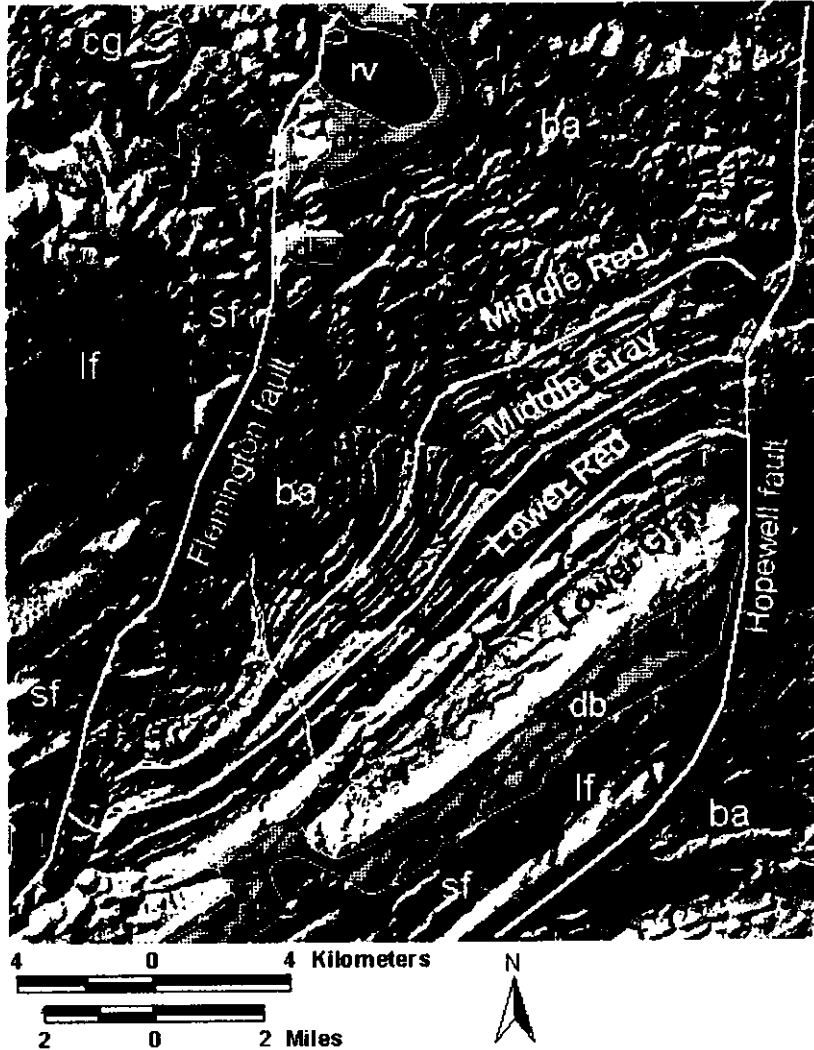
Figure 3. Shaded relief map of the area between Round Valley reservoir and Sourland Mountain in the central part of the Newark Basin, New Jersey. The regional hydrostratigraphic units of the Brunswick aquifer correlate with pronounced topographic ridges and illustrate how the distribution of bedrock influences topographic relief. db –diabase, sf – Stockton Formation, lf – Lockatong Formation, ba- Brunswick aquifer, cg – conglomerate, rv – Round Valley reservoir.
