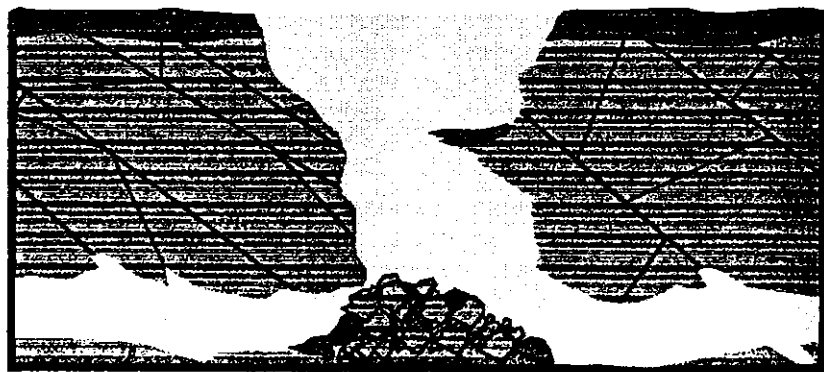
Figure 3B - Cave Collapse Sinkhole
