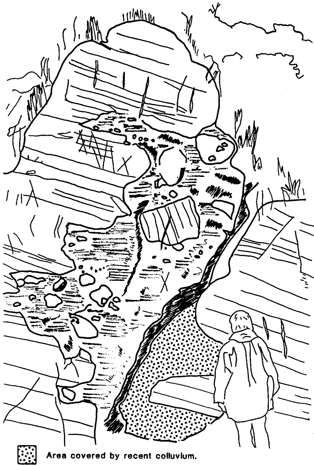
Figure 8. Line drawing (from photograph) showing paleosinkhole in Alpha, New Jersey. Infilling of eroded area interrupts bedding dipping from upper left to lower right.
